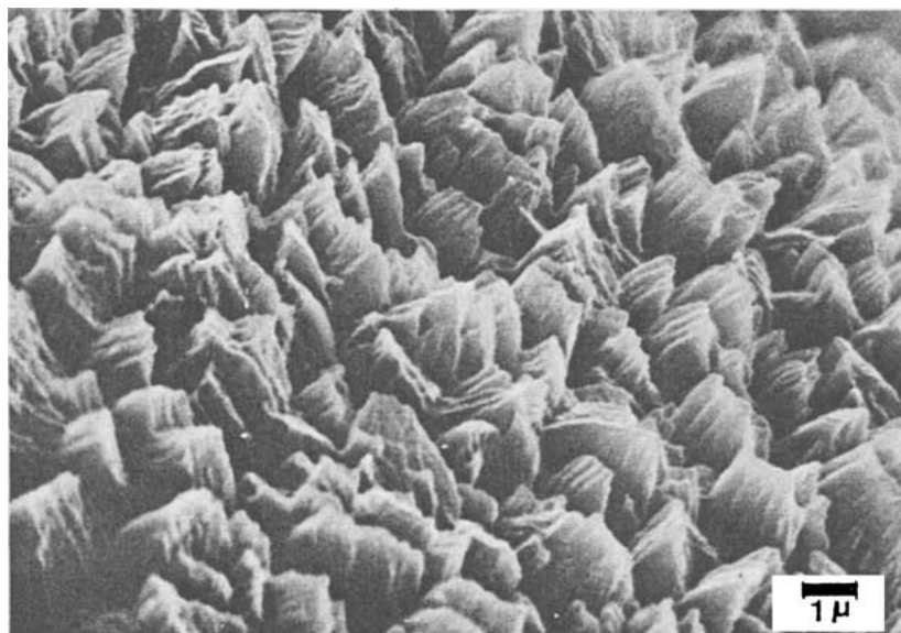
Figure 15 SEM micrograph of faceted interfaces of isotactic polypropylene highlighted by ion-bombardment after crystallized from the melt. (Courtesy of M. Kojima).
