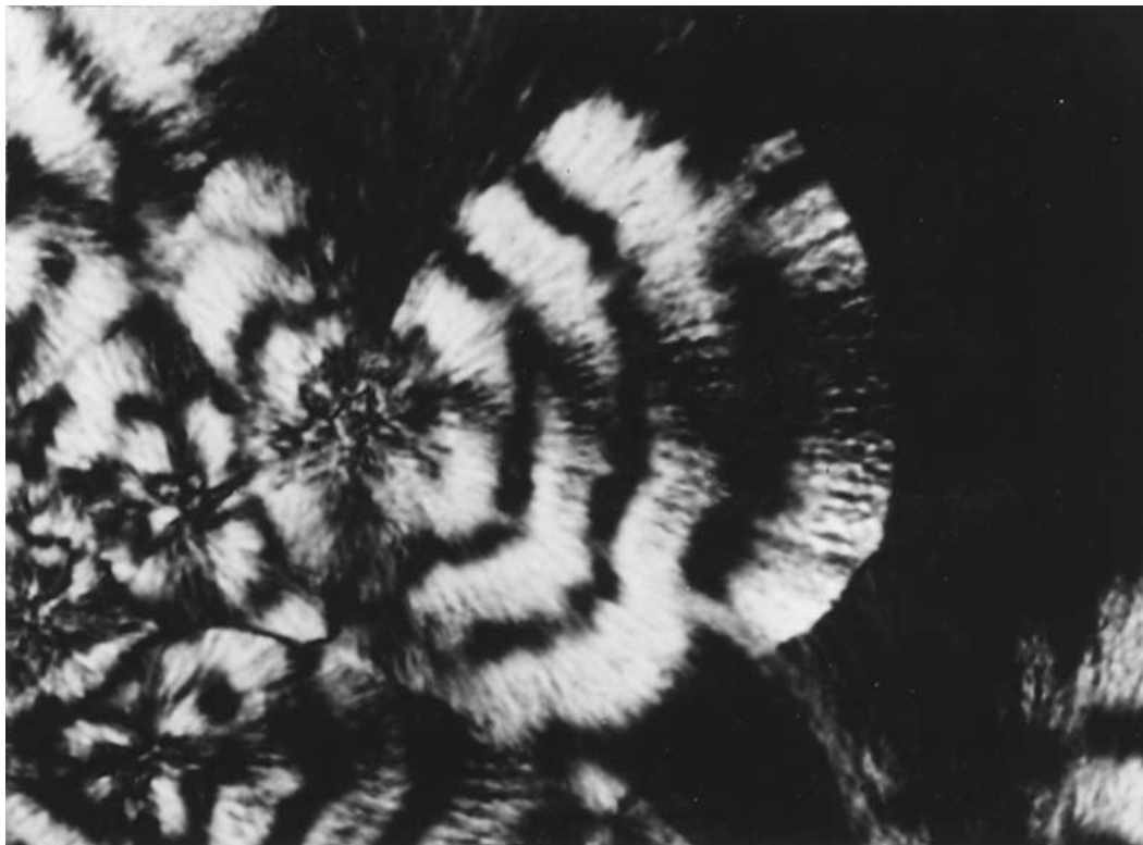
Figure 12 Melt crystallized nylon 7.7 spherulites with 50 \mu\text{m} spacing crystallized isothermally from the melt at 187°C after fusion at 260°C (30 min.) (unpublished).
