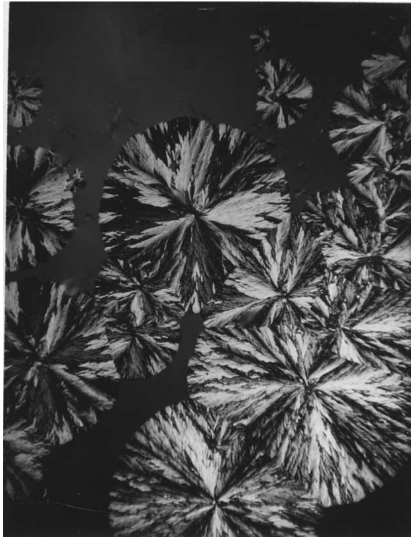
Figure 1 Floreal-looking nylon 4,9 negatively birefringent spherulites crystallized from the melt at 235°C (16 hr). Fusion temperature 267°C (1/2 hr); \times 128 .
